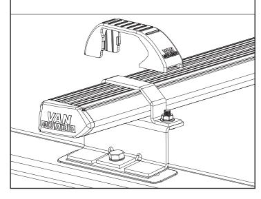
Remove roof bars leaving only the existing roof brackets fixed to the vehicle.
