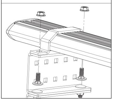
Once in position tighten all fixings to 8Nm. Periodically check all fixings.
