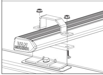
Secure the roof extension brackets onto the existing roof brackets using M6x16 coach bolts & M6 serrated nuts.
