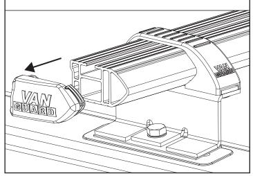
Slide the rail plates into t-slot of the roof bar and fit the newly supplied end bung.
