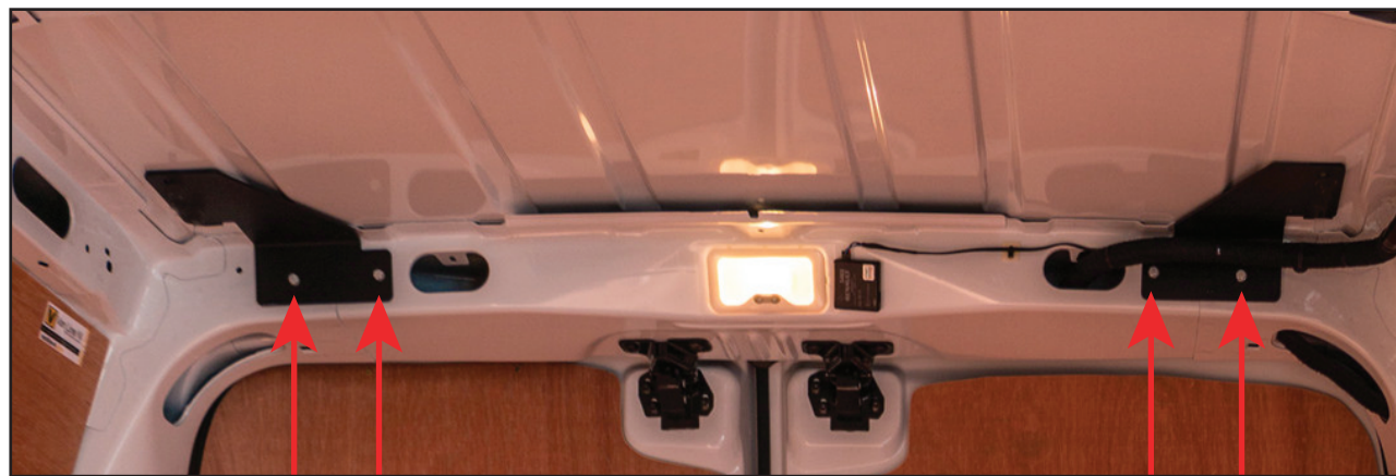
M6 1/4 TURN NUT INSERT LOCATIONS
