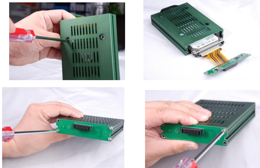
Figure 10 Open the hard disk case
