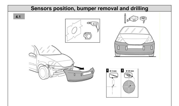
Use a paper tape to mark the positions of the sensors holes on the bumper.
