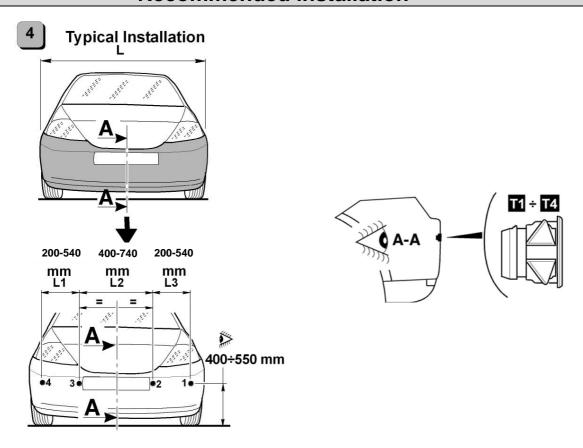
Installing the sensors within the following range:  $L1=\min 200-\max 540 \text{ mm}-L2=\min 400-\max 740 \text{ mm}-L3=\min 200$  -  $\max 540 \text{ mm}$ , usually it is not necessary to perform the central unit configuration procedure. After having installed the system, we suggest you, to perform a functional test, if the test result is negative, it is necessary to perform the central unit configuration procedure. (Chapter 1.3 and 12.4).
