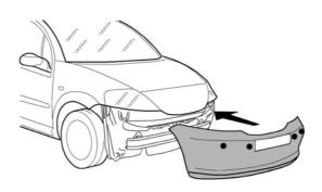
After having performed the sensors connections, reassemble the bumper on the vehicle, paying attention to the wires.
