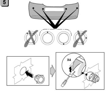
The sensors must be inserted in the bumper with the reference mark upwards. They can be rotated 180° degrees without compromising the proper functioning. Check that the fixing wings are correctly opened, otherwise open them using a small screwdriver as shown in the picture.
