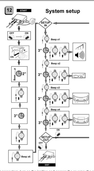
Disconnect J2 and J3 connectors, turn on the ignition and engage the reverse; the system beeps sounds for 2 s, disconnect and reconnect the connector of the loudspeaker to enter in the programming procedure, the system beeps 6 times.
