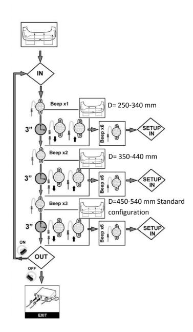
The system beep once indicating the sensors distance of 250-340 mm, after 2 s beeps 2 times indicating the sensors distance of 350-440 mm and after other 2 s beeps 3 times indicating the sensors distance of 450-540 mm. To choose the desidered distance, disconnect and reconnect the connector after hearing the number of beep selected. When the loudspeaker connector is reconnected the system store the selected distance choice and goes back to the main menu beeping 6 times.
