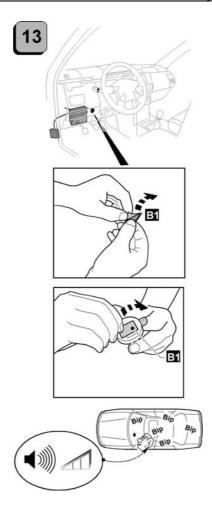
Test the loudspeaker volume before fixing it. Put an obstacle in front of the bumper and turn the ignition on or engage the reverse gear. The loudspeaker beeps: check if the sound is well audible for the driver (with the engine running). If the sound level needs to be adjusted, perform the procedure of chapter 12.1. After checking, remove the protective film of the B1 biadhesive and fix it.
