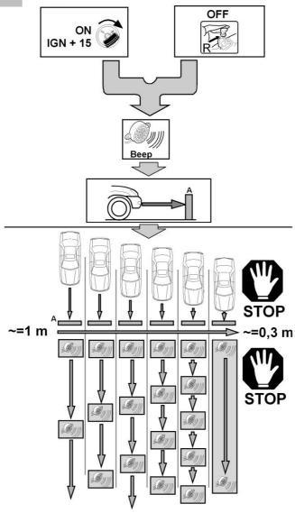
Position the vehicle with the sensors facing a wall at a distance of approximately 1 mt, turn the ignition on and engage the reverse gear. The system confirms its activation with 1 beep. Get closer to the wall at a low speed. The beeps frequency increases getting closer to the wall.
