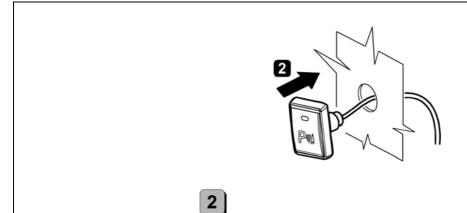
Insert the wiring and install the pushbutton.
