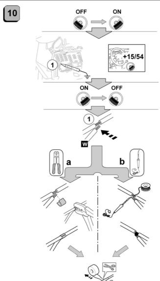
To identify the ignition key (+15/54) wire, it is necessary to turn the ignition on and check with the test lamp. Turn off the ignition, connect the Green-Red (W) wire to the ignition wire by crimping or soldering it. Isolate the junction with tape.
