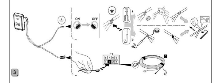
Connect the wire without terminal to ground and insert in position 3 of the J1 power supply connector the fastoned wire.
