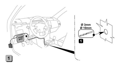
To make a hole of 3 mm and then 10 mm in the chosen location for the installation of the pushbutton.
