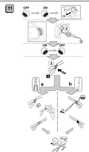
To identify the reverse wire, it is necessary to turn the ignition on , engage the reverse gear and check with the test lamp. Turn off the ignition, connect the RED of the main harness wire by crimping or soldering it. Isolate the junction with tape.
