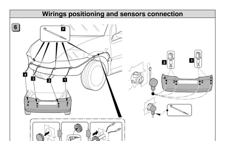
Use an original grommet to route the sensors wirings out of the vehicle.
