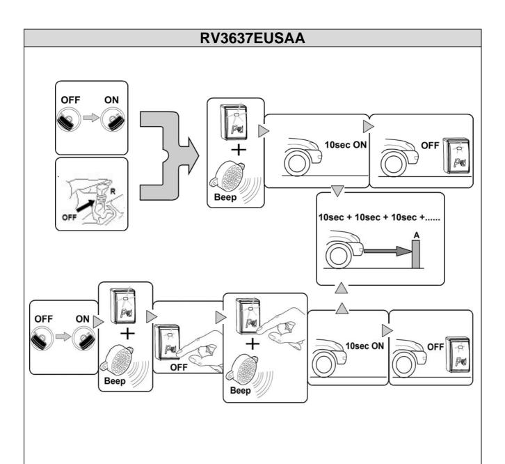
The system is activated at the ignition on , if not detects obstacles within 10 s is deactivated.
