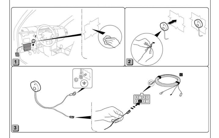
Clean the chosen location to install the pushbutton, remove the protective film of the biadhesive and fix it. Connect the black wire with ring terminal to ground. Insert in position 3 of the J1 power supply connector the fastoned wire.
