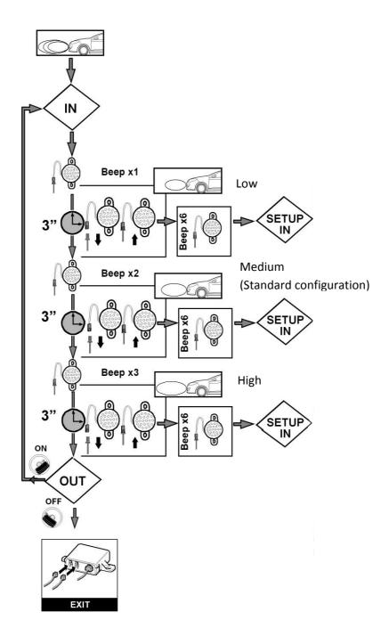
The system beep once indicating the low sensitivity, after 2 s beeps 2 times indicating the medium sensitivity, after other 2 s beeps 3 times indicating the high sensitivity. To choose the desired sensitivity, disconnect and reconnect the connector after hearing the number of beep selected. When the loudspeaker connector is reconnected the system store the desired sensors sensitivity and goes back to the main menu beeping 6 times.
