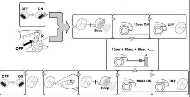
The system is activated at the ignition on , if not detects obstacles within 10 s is deactivated.
