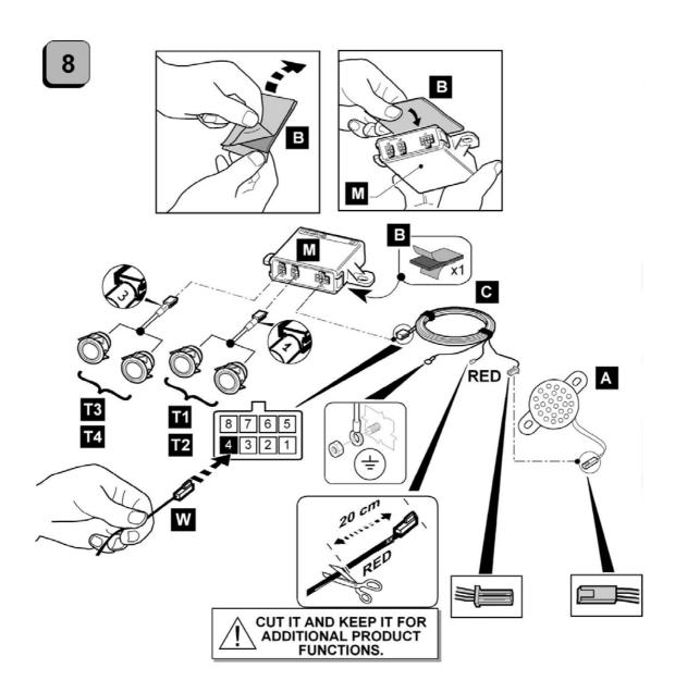
Use the B biadhesive to fix the central unit. Connect the connector marked 1 in J2 position and the connector marked 3 in J3 position of the central unit.
