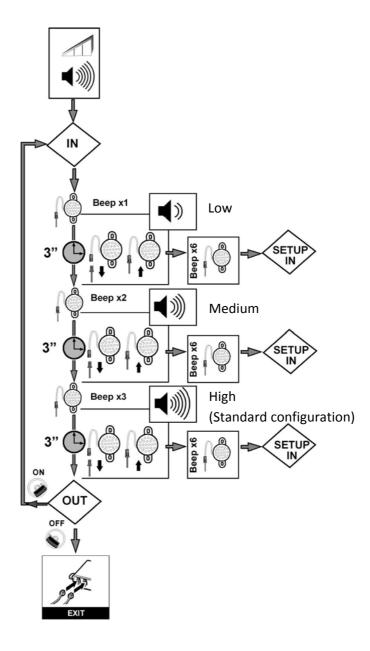
The system beeps once indicating the low volume, after 2 s beeps 2 times indicating the medium volume and after other 2 s beeps 3 times indicating the high volume. To choose the desired volume value disconnect and reconnect the connector after hearing the number of the beep you want to select. When the loudspeaker connector is reconnected the system memorizes the desired volume and goes back to the main menu beeping 6 times.
