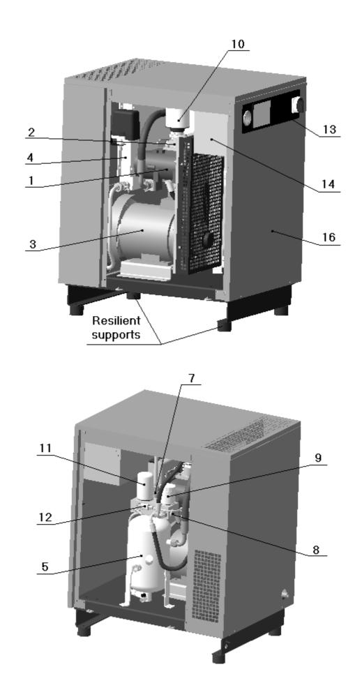
Figure 1 – The general view of the compressor unit BK5E-..., BK7E-..., BK10E-...
