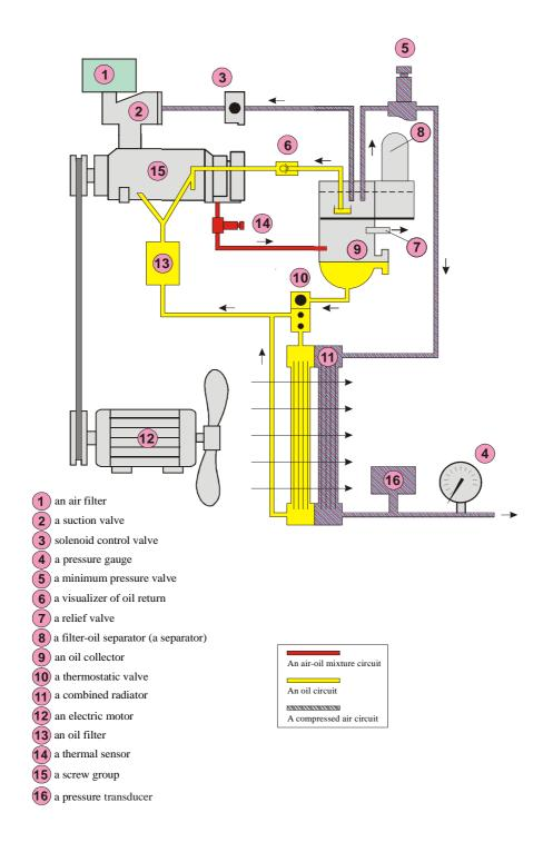
Figure 7 – Functional circuit diagram of the compressor unit BK5E, BK7E, BK10E
