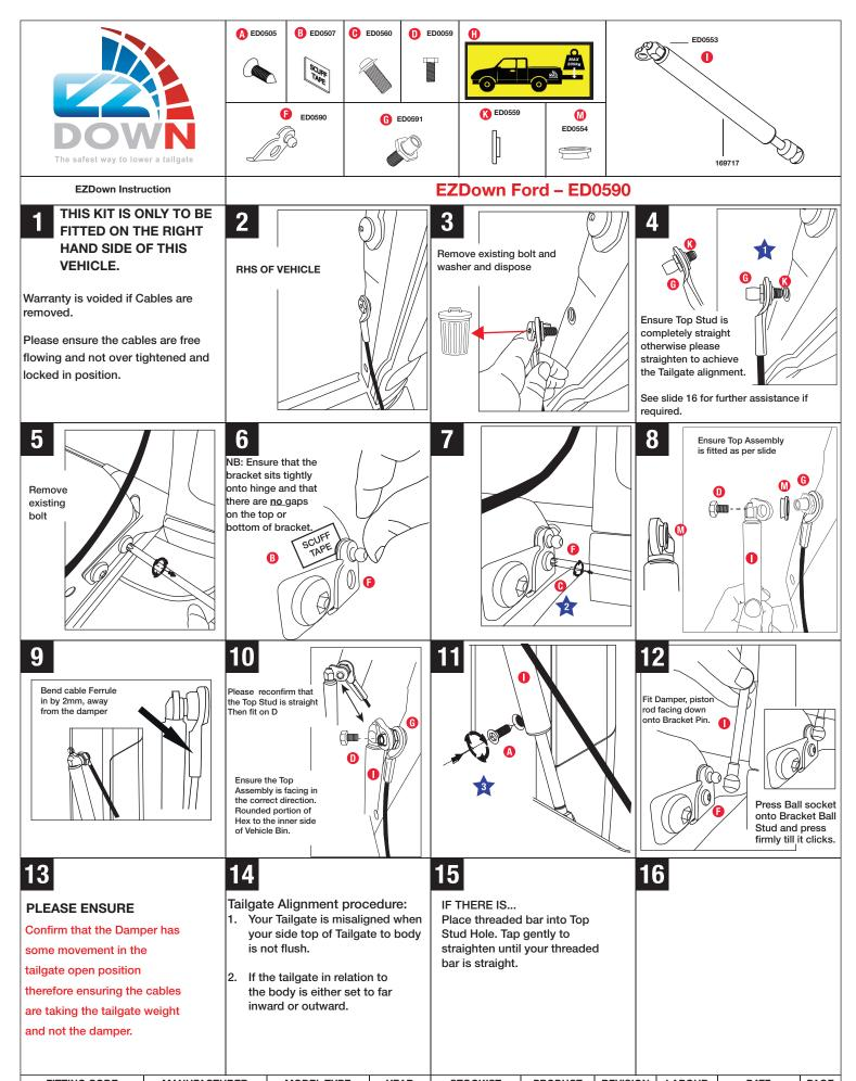
FITTING CODE MANUFACTURER STOCKIST PRODUCT REVISION DATE MODEL TYPE YEAR LABOUR PAGE 2011 ED0590 **FORD** FORD T6 **GENERAL USE EZDown** 20min 01/07/2019 1 onwards TORQUE - N.m 25N.m ± 2N.m 17N.m ± 2N.m OUDLY SOUT 65N.m ± 2N.m www.ezdown.co.za
