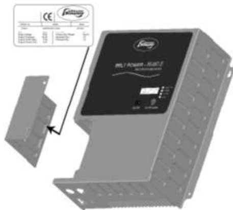
Fig. 2: Identification plate inverter box.
