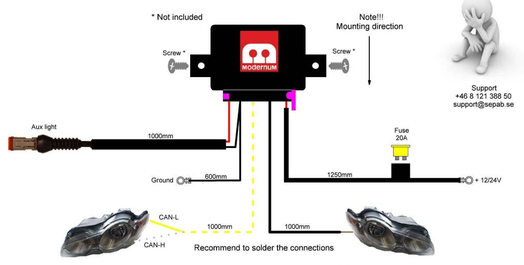
Note! White (CAN-H) and yellow (CAN-L) twisted cable;  $\underline{\text{Digital}}$  signal in.
