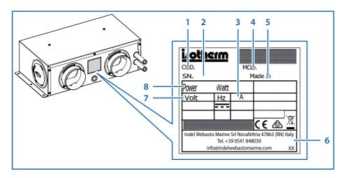
It contains the model, serial number and all the technical data of the product necessary to request spare parts or to report technical problems to the service centre.
