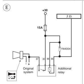
Vehicle horn connection with additional relay.
