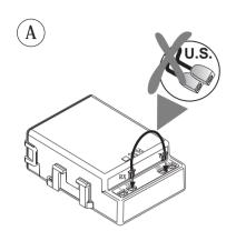
Install the jumper wire (see the catalogue) between the Ultrasound TX and RX, if you don't use the volumetric sensor.
