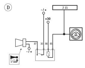
Original relay controlled by a negative signal. Vehicle horn connection with negative control signal to the original relay.
