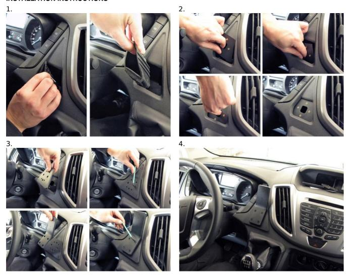
Please read the instructions and look at the pictures carefully before installing the mounting bracket. This product consists of three parts:
