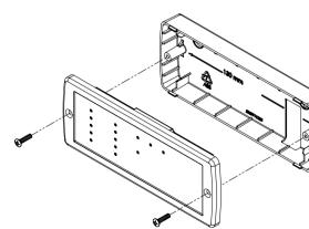
When the remote control is mounted on the dashboard, the back cover can be used as drill guide.
