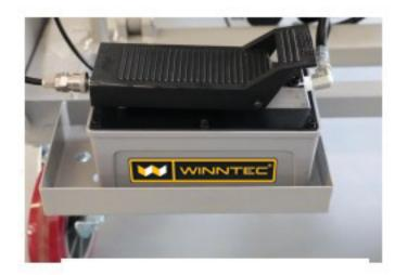
Hydraulic pneumatic pump drive
