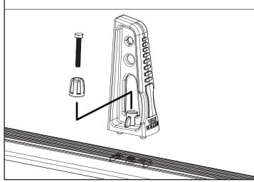
Slide the load stops to the required position on the bar and then tighten by hand.
