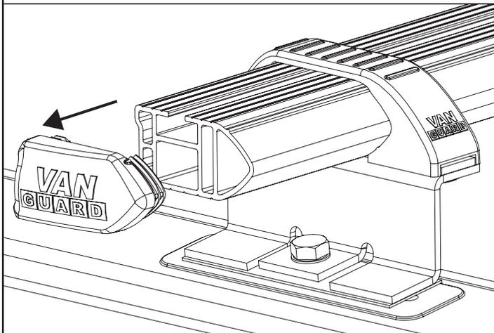
**2** Slide the rail plates into t-slot of the roof bar and fit the newly supplied end bung.
