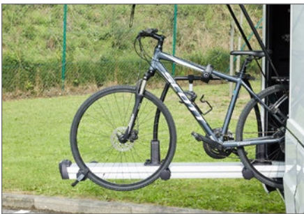
[1] Bike rack slides out up to 1.50 meter
