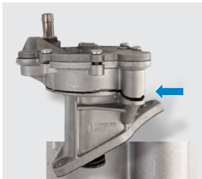
Fig. 1: Breakage in the pump housing
