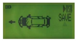
The display shows a vehicle pictogram. The up/down keys on the device can then be used to select the tyre you wish to read out. This also includes the spare tyre.
