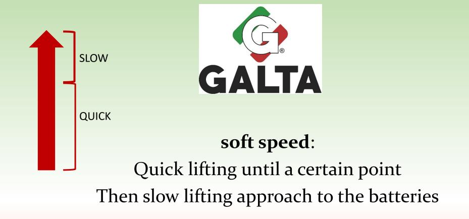
This way you can be sure **not to damage the batteries** or sensible parts
