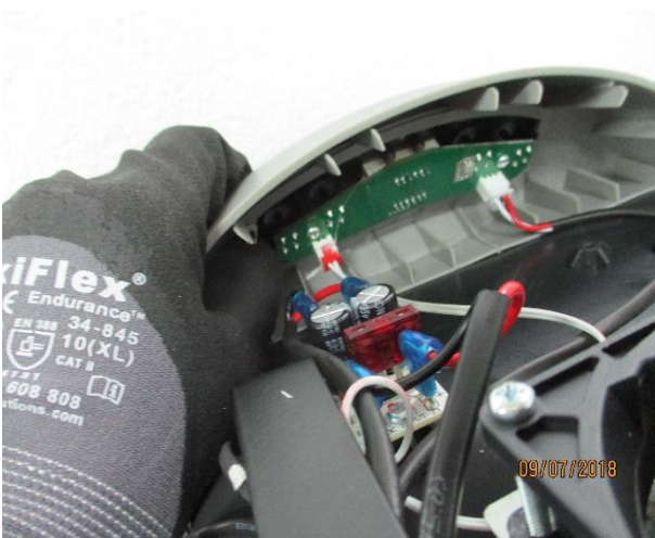
4. Press on the display's corner to remove it
