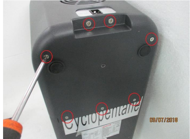
2. Unscrew the screws fixing the cover (7 screws)
