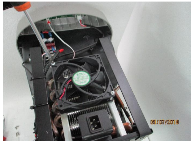
4. Unscrew the 2 screws fixing the fan, disconnect the wires connecting the fan and the ECU and reverse the procedure to replace it
