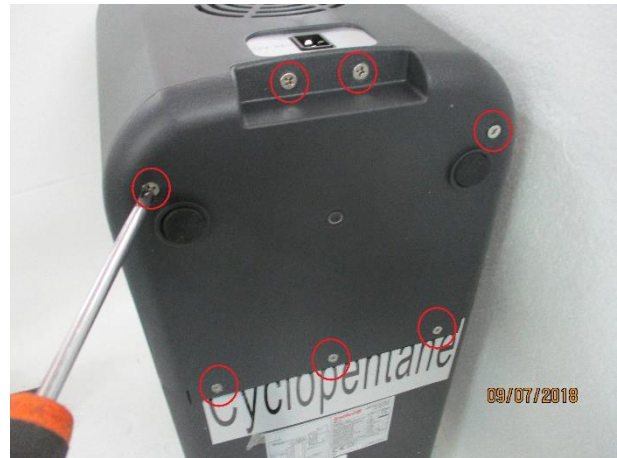
2. Unscrew the screws fixing the cover (7 screws)
