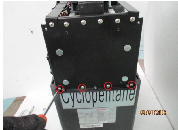
4. Unscrew the 4 screws fixing the metal base
