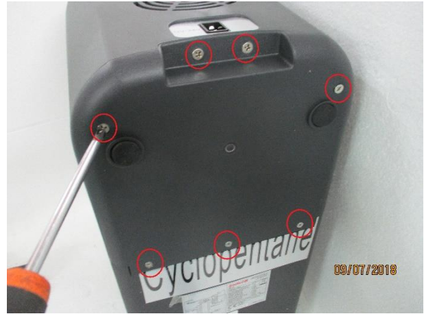
2. Unscrew the screws fixing the cover (7 screws)
