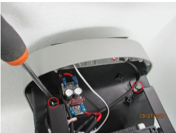
5. Unscrew the 2 screws fixing the 2 brackets
