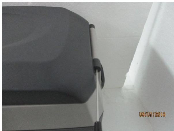
2. Insert an awl in the small holes to remove the lid
