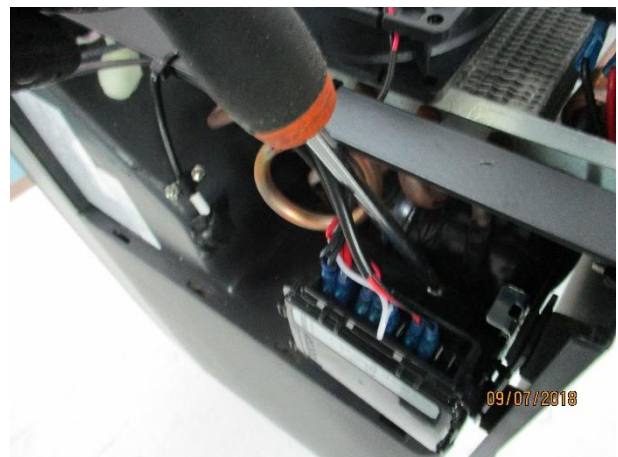
6. Unscrew the screw fixing the ECU
