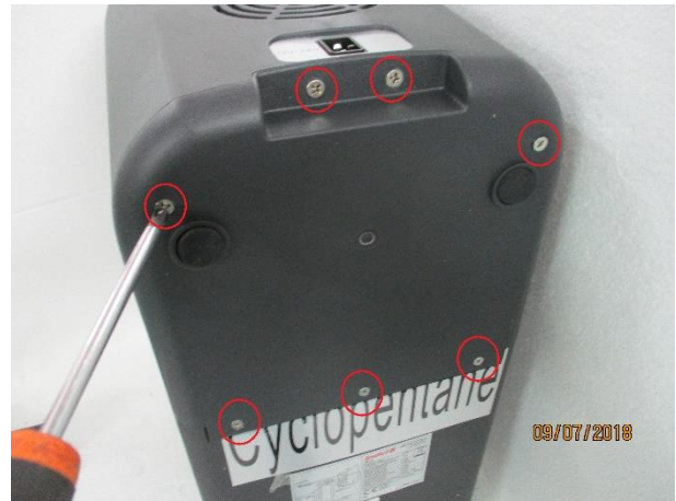
2. Unscrew the screws fixing the cover (7 screws)
