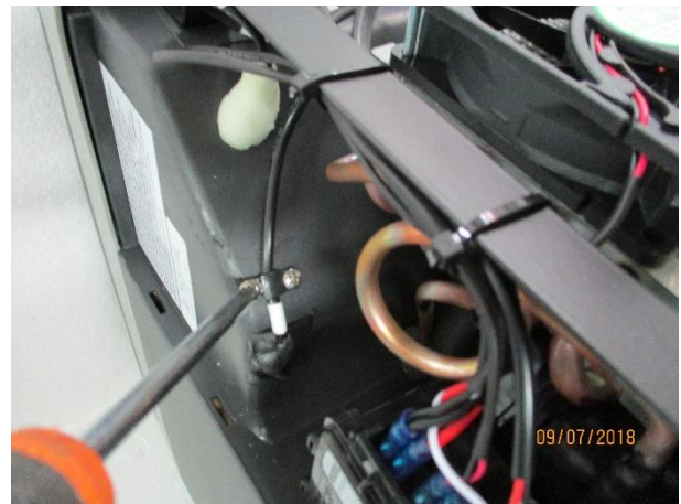
4. Unscrew the 2 screws fixing the sensor
