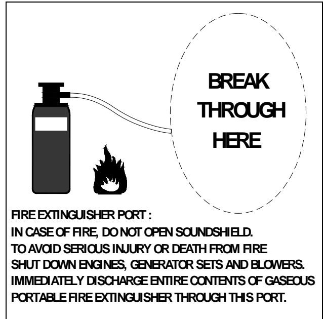
Fig. 3 Fire extinguisher port.
