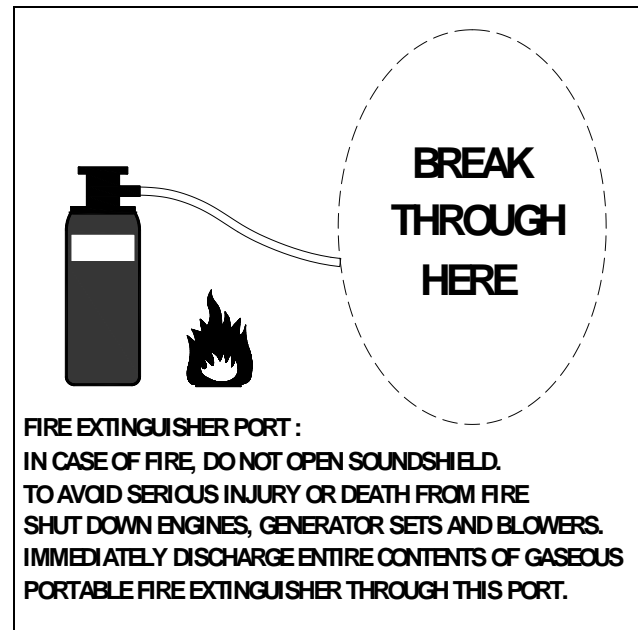
Fig. 2: Fire extinguisher port.
