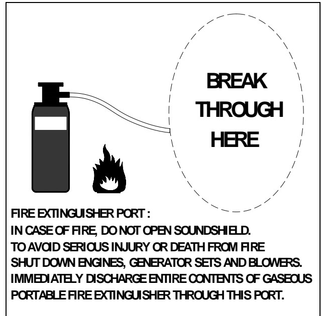
Fig. 2: Fire extinguisher port.
