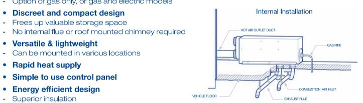
Underfloor Installation VEHICLE FLOOR -\_\_\_\_ COMBUSTION AIR INLET
