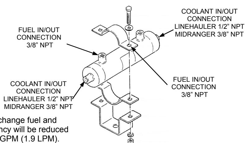
**CAUTION:** While it is physically possible to interchange fuel and coolant connections in pairs, heat transfer efficiency will be reduced by up to 43% on fuel systems which flow over .5 GPM (1.9 LPM).
