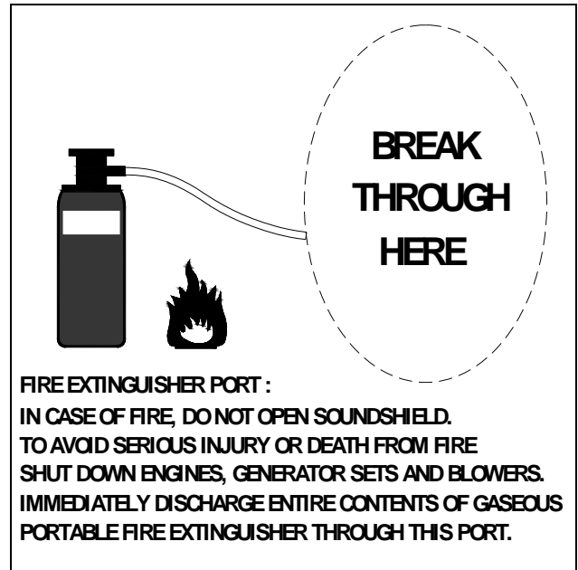
Fig. 2: Fire extinguisher port.
