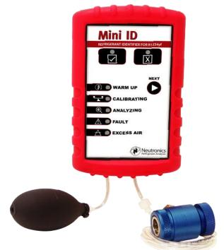
A "GREEN" PASS LED is illuminated for R-1234yf purity greater than 95% while a "RED" FAIL LED is illuminated for R-1234YF with a purity of less than 95%.
