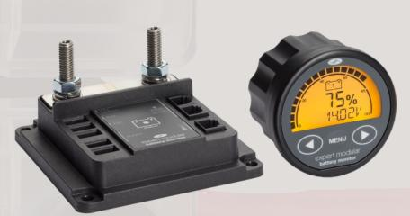
The Expert Modular can monitor up to three battery banks. The inputs for battery bank 2 and 3 can also be configured for other purposes, like mid-point voltage measurement, keyswitch input, setup lock or backlight control. The Expert Modular battery monitor can measure DC currents up to 600Amps (500Amp continuous) and voltages up to 70Vdc. So any lead- or lithium based battery from 12V up to 48V can be monitored.
