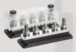
All DC Modular products are equipped with stainless steel studs, washers and nuts for optimal corrosion resistance. Tin plated high purity copper busses provide maximum conductivity, reducing heat and improving efficiency. The base material used for the DC Modular products is made from a special, fiber reinforced compound. This material offers excellent high temperature properties, good chemical resistance and high strength.
