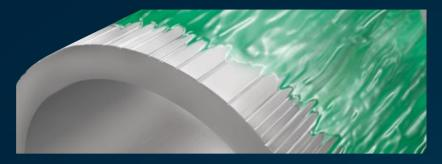
Metal tubes can have longitudinal grooves on the surface from production. These production-related faults can be compensated quite easily by moistening the tube ends to be connected with LOKPREP fluid before assembly. Thanks to its capillary characteristic, it can even flow into microscopic cavities and fill these out completely. LOKPREP is not an adhesive, rather an anaerobic sealant which hardens under oxygen exclusion and in contact with free metal ions.
