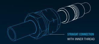
You can use these connections together with LOKRING or LOKCLIP connectors to replace faulty threads. If you should damage a thread during servicing (e.g. while replacing a condenser), it is no longer necessary to replace the whole tube. You can simply repair this again with the O-ring repair connections.
