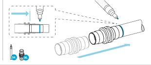
Choose the correct LOKPREP (05) for the tube material and the ambient temperature.
