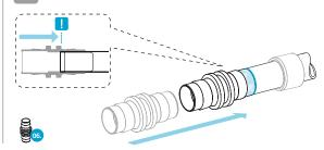
Put the assembly jaws (08) in place behind the LOKRING (07) and the assembly stop of the joint (06). Press the tube connection together. Do not change the insertion depth of the tube and joint (06). Press the tube connection until the LOKRING (07) is flush to the assembly stop of the joint (06). Respect the curing time of the LOKPREP (05) before applying forces to the connection.
