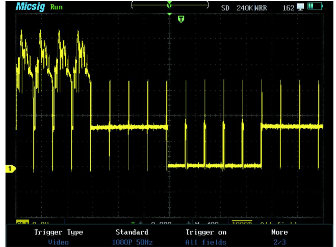
Support various video triggers, PAL,NTSC,SECAM,720P,1080I,1080P
