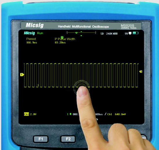
Three operation modes for moving waveform, zooming in and out, and using menu by touch, button and scroll wheel.
