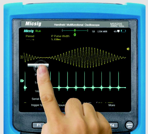
Three operation modes for moving waveform, zooming in and out, and using menu by touch, button and scroll wheel.
