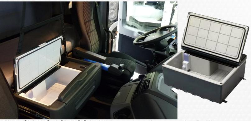
MERCEDES ACTROS MP3 is equipped as standard with a drawer in which is possible to install TB025AM which fits perfectly as the genuine one! A fridge for NEW ACTROS MP4 is under development.
