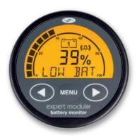
When an alarm is activated (for example due to a low battery state of charge), the alarm bell icon will be lit and an explanation about the type of alarm will scroll through the display. An audible alarm can be enabled to let the CDU beep for additional attention.
