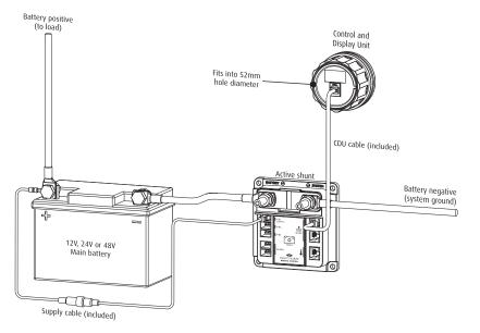
Example schematic of a single battery setup. Notice the small amount of cables that are needed to get the Expert Modular up and running. The supply and CDU cables are both included. Also included but not shown in the above picture are rubber caps to cover unused I/O ports against polution.
