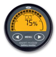
The image on the left shows the normal operating mode with the second parameter row disabled. This results in a clean display area that only shows the battery state of charge (%) and the bar graph. A perfect mode for less technical end users.
