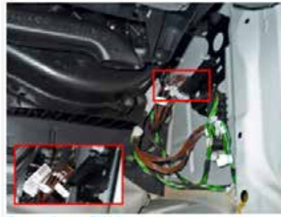
Connection to CAN A Connection to CAN A behind the right side panel in the passenger footrest.
