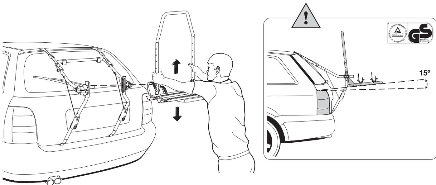
**EN** Select the right height and holes for installation. The platform should not obstruct the rear lights or number plate.
