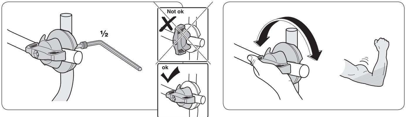
**EN Check the tension.** After a period of use, it may be necessary to check the tension in the knob. Tighten the hexagonal screw half a turn and check that there is greater resistance in the knob when you turn it. **NOTE:** The knob should always be in the tensioned setting.
