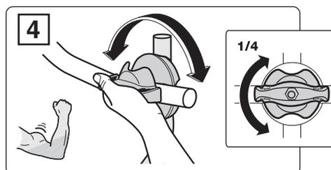
**EN** 1. Fit the knob as in the diagram. 2. Tighten the screw until it is no longer possible to undo the knob by hand. 3-4. Loosen the screw 1/2 a turn at a time until it is possible to turn the knob by hand (**the knob should not move easily when it is loosened**).
