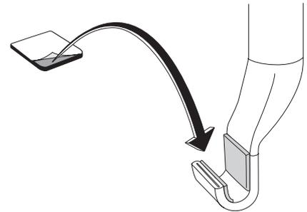
**EN** Check that the hooks remain free when shut. If the lower hooks strike the bumper, the rubber protector can be split and fitted on the sides of the lower hooks.
