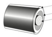
Plastic vinyl Hardened steel link rings Ultra hard steel cable
