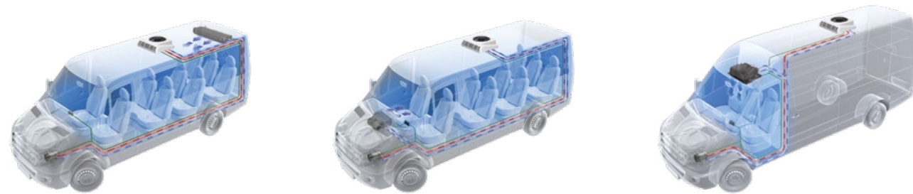
Evaporator under the roof Evaporator under the dashboard Evaporator integrated into the roof
