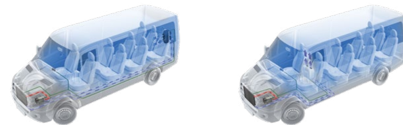
Evaporator vertical on the side at the rear Evaporator vertical
