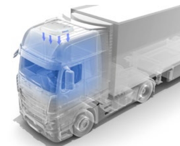
Parking air-conditioning system
