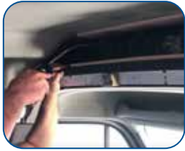
Leak in evaporator in an ambulance.
