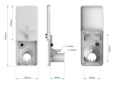
Unique 2 in 1 design includes a 12V pump power supply and Onboard Tank Fill all in one socket. The secure hose clip keeps the pump in place during filling. The Onboard Tank Fill + 12v Power Socket incorporates a lock to protect your water supply and a vent pipe ensuring the tank is vented at all times, preventing airlocks. This socket is suitable for use with any standard hose and is to be used with cold freshwater only.
