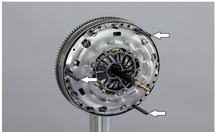
Fig. 2: Stud bolts for holding the spindle carrier
