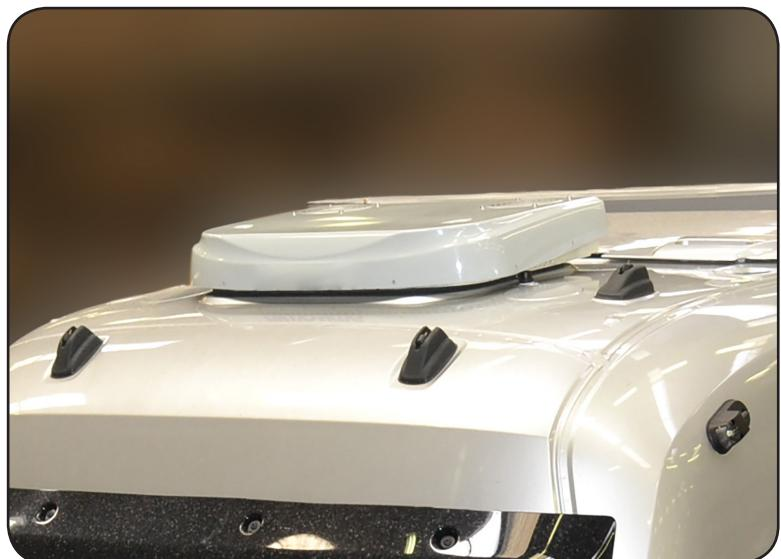
Fix the air conditioner using the brackets **B**: insert the ends of the brackets under the lining to gain a grip on the metal parts; insert screws **CC** with the washers **DD** and nuts **EE** and screw them into the threaded sockets on the bottom of the air conditioner. Tension and then tighten the nuts **EE** against the brackets **B**.
