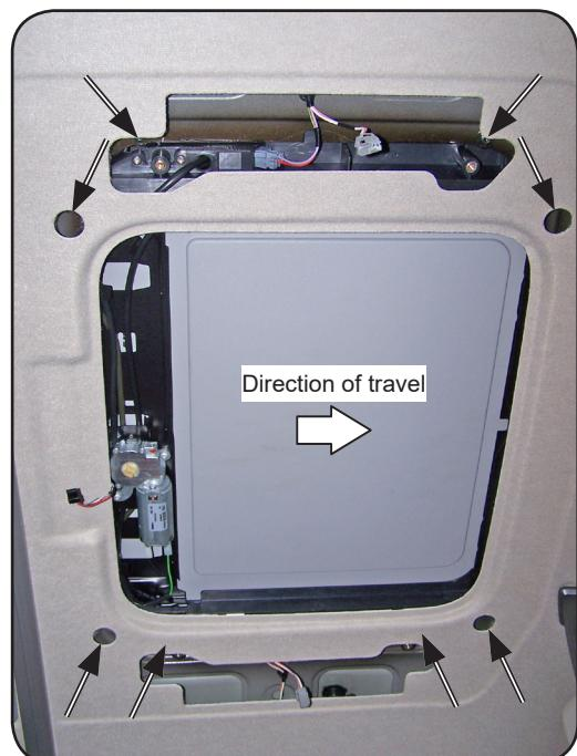
Spread sealant along the edge of the hatch opening where the air conditioner gasket will be placed.
