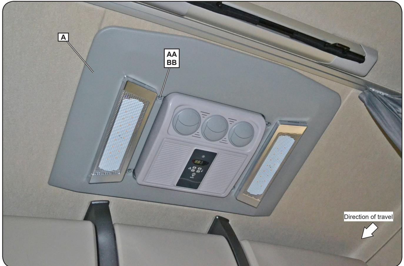
Refit the ceiling lights on the new panel.
