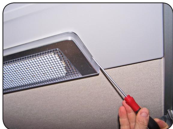
Remove the internal cover panel from the hatch and discard it.
