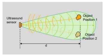
Picture 2: Ambiguity: Ultrasonic sensors can measure the distance to an object by timing the reflection of sound waves, but they cannot determine the object's direction or velocity. The object can therefore be at several different positions in the field of view
