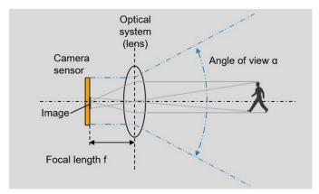
Picture 1: How a digital camera works: The optical system projects an image of the environment onto the sensor. The area covered by the image depends on the focal length and the angle of view.
