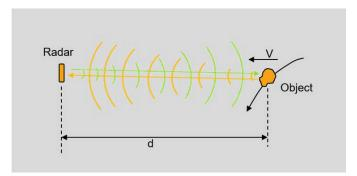
Picture 3: How radar measurement works: Radio waves are reflected by objects, and the reflection time allows their distance to be calculated.
