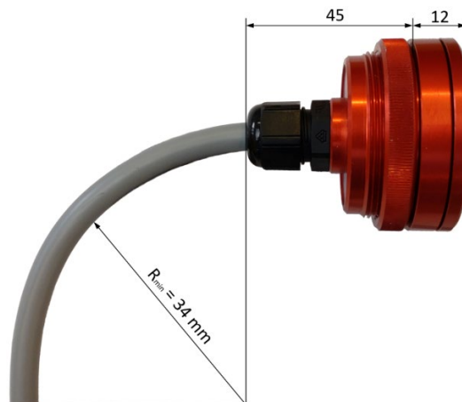
Minimal cable bending radius
