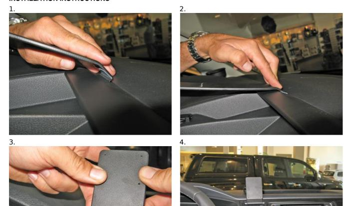
Please read all of the instructions and look at the pictures before installing the ProClip. Important! This ProClip will cover the 12V socket on top of the dash, there will be approximately 40mm between the socket and the ProClip. The ProClip can also be placed on the right airvent.
