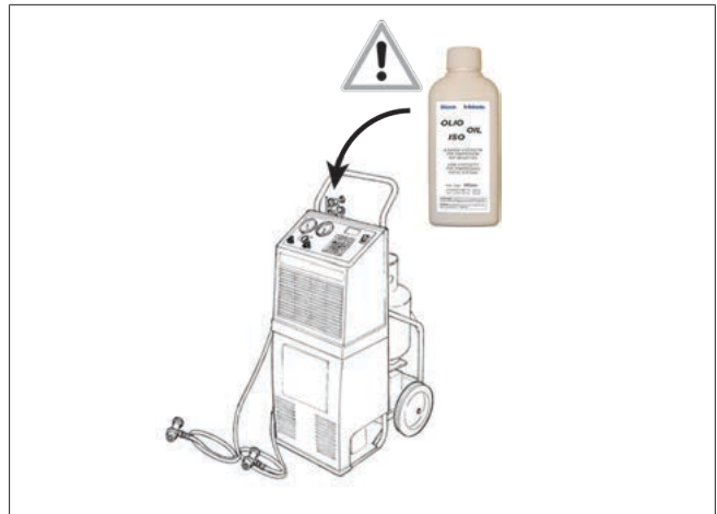
Fig. 8 Add the correct quantity of lubricant
