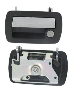
This flush mounted paddle is a redesign of our 030-0450 paddle handle for compartment doors and entrance doors on recreational and specialty vehicles. Containing the same proven mechanical details as previous with a modernized look, it can be used in FMVSS 206 applications, is power lockable and features two point remote pivot plate and lock cam actuation.
